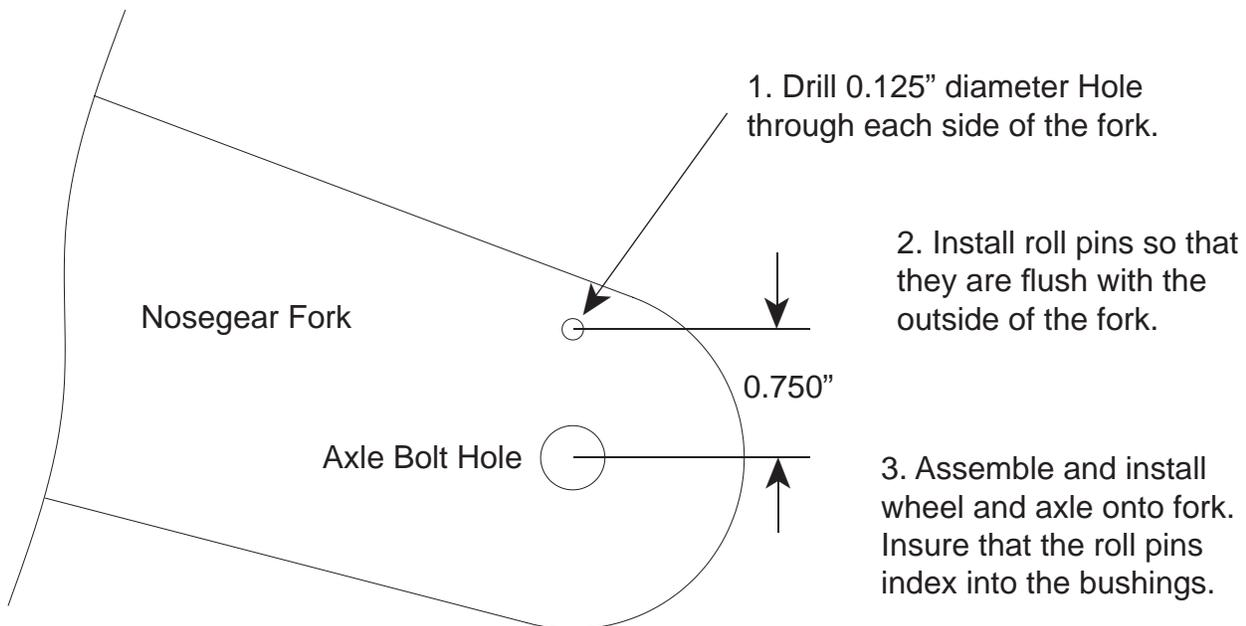
4. Tighten axle bolt and observe wheel drag. If wheel has side play or spins freely with no wheel bearing drag, disassemble and trim inner sleeve just enough to eliminate all side play and achieve a slight wheel bearing pre-load drag when the axle bolt is tightened.
