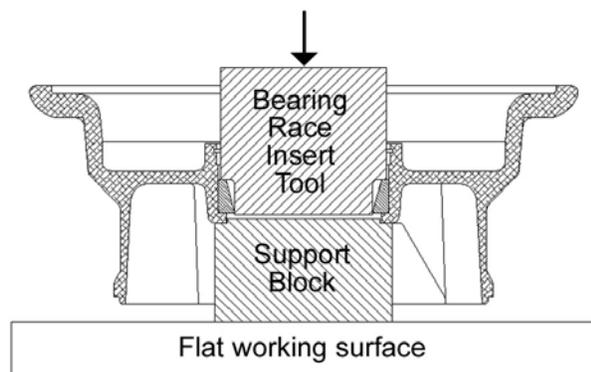
in breakage of the wheel casting if too much force is applied.
